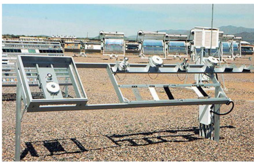
**One of several solar radiation monitoring racks at Atlas' DSET Laboratories in Phoenix, Arizona. Detailed field solar radiation data is often used when comparing laboratory exposure "equivalents."**
