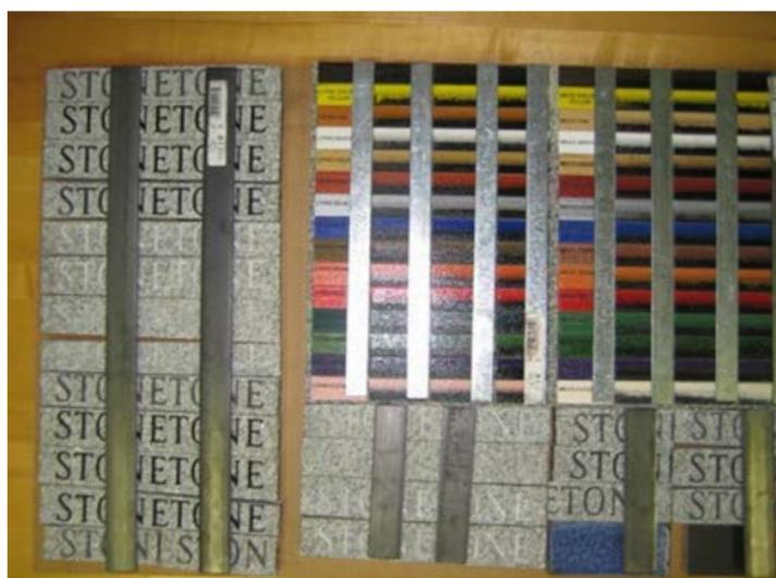
Figure 2. Test specimens (post exposure) of the imaged granite; steel bar masks provided non-irradiated areas for visual comparison.
