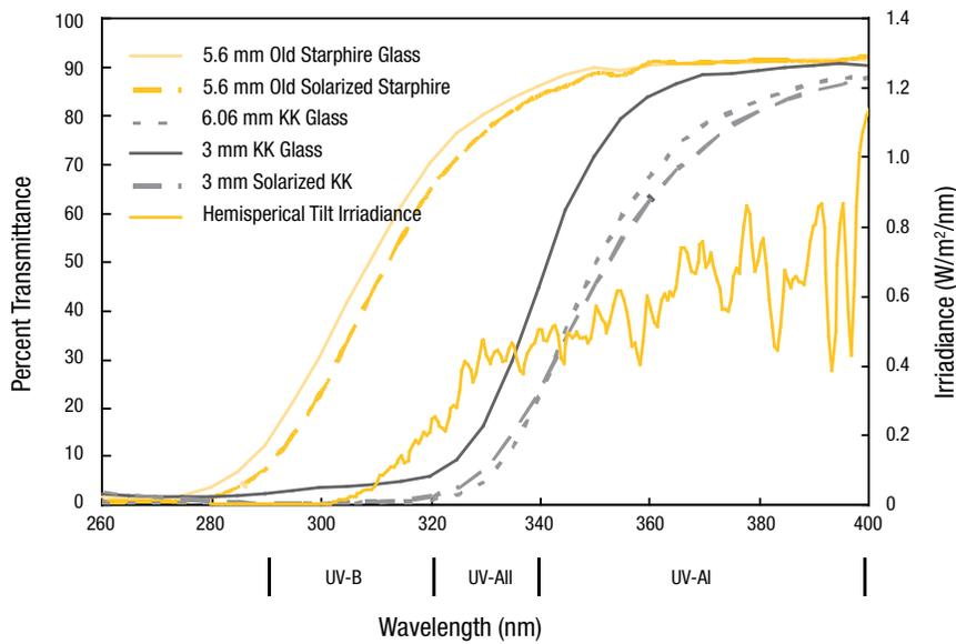
**Figure 2.** UV light transmission through a variety of glass samples plotted along with the AM 1.5 spectrum for comparison. Samples labeled “solarized” had been exposed to 114 W/m<sup>2</sup> (300 nm to 400 nm) in a Ci4000 Weather-Ometer® at 60°C and 60% RH.
