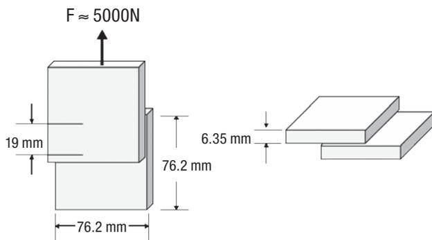
Figure 1. Schematic of lap shear samples.
