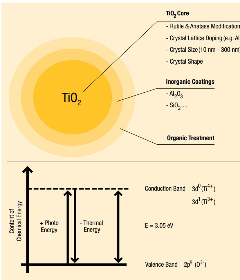
**FIGURE 2:** Ultra-fine titanium dioxide is being modified for UV absorption without photocatalytic activity: doping, inorganic and organic coatings UV absorption triggers the transfer of an electron from the valence band to the conduction band. The absorbed energy is released as harmless radiant heat.
