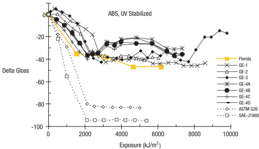
**Figure 6.** ABS containing carbon black tested repeatedly under new GE conditions, G26, J1960, and Florida (with correlation factor of 1 year=3100 kJ/m<sup>2</sup>/nm at 340 nm).
