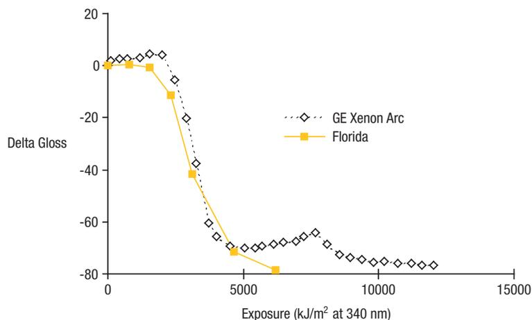
**Figure 4.** Superposition of Miami data on xenon arc data for a sample of white ASA/PC blend using a shift factor of 3100 kJ/m<sup>2</sup>/nm (340 nm) per year of Miami exposure.
