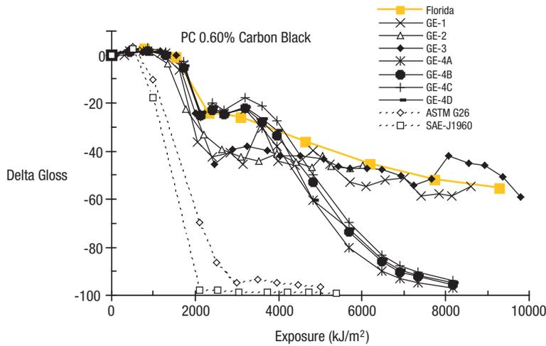
**Figure 5.** PC containing carbon black tested repeatedly under new GE conditions, G26, J1960, and Florida (with correlation factor of 1 year=3100 kJ/m<sup>2</sup>/nm at 340 nm).
