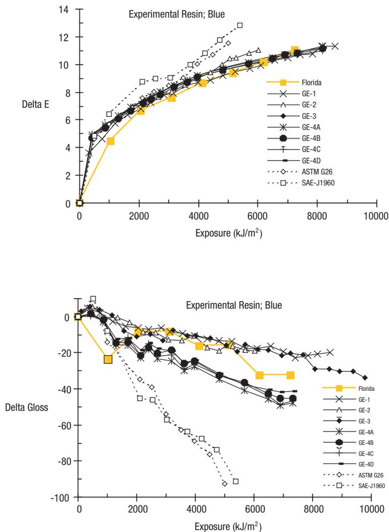
**Figure 7.** Color shift and gloss loss for a blue experimental resin tested repeatedly under new GE conditions, G26, J1960, and Florida (with correlation factor of 1 year=3100 kJ/m<sup>2</sup>/nm at 340 nm). Both colorant and resin undergo a color shift.
