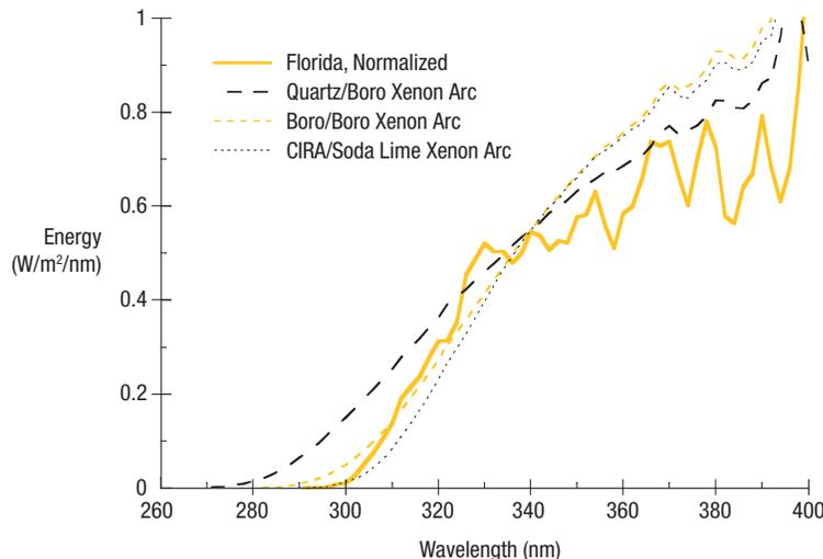
**Figure 3.** Spectral distribution of light sources.
