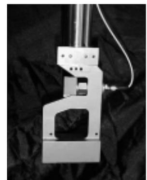
Instrumented Charpy Pendulum
