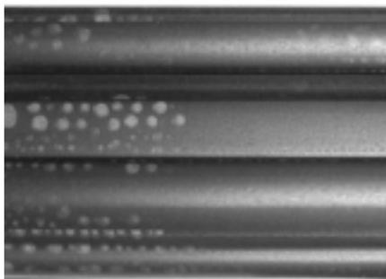
*Photo of coated rubber sample after weathering testing in an Atlas Weather-Ometer®.*
