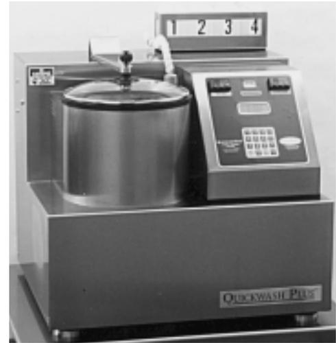
*The Quickwash Plus accelerates testing for determining dimensional stability or shrinkage of fabric.*
