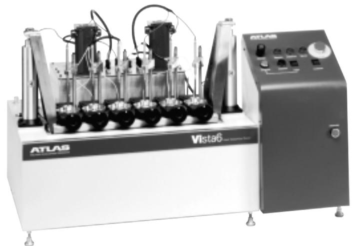
*The Atlas Vista6 Heat Distortion Tester will make its debut in June at NPE 2000.*
