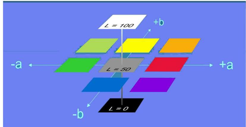
**Figure 4.** CIE L\*a\*b\* value defines a color by its 3-dimensional coordinates on this scale.
